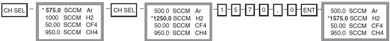
The example above shows how the setpoint for Channel 2 is changed. When **CH SEL** is depressed an asterisk points to the channel selected. To select Channel 4, depress **CH SEL** switch 4 times. The value displayed after the asterisk is the current setpoint value. Typing in a new value overrides the old value. If **ESC** is depressed instead of **ENT**, the old value is retained.
