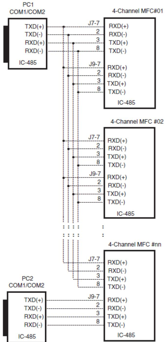
RS232/485 data is transmitted at 9600 or 19.2K baud (user-selectable) in the following format:
