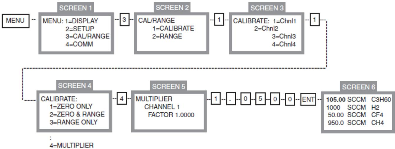
Entering a MULTIPLIER value changes the display by that multiplier factor. All data values are multiplied by the MULTIPLIER prior to display. The MULTIPLIER is sometimes referred to as a GAS CORRECTION factor when used with MFC's. If the MFC is calibrated with nitrogen and another gas is used with the MFC, a GAS CORRECTION factor can be entered to recalibrate the MFC to the gas used.
