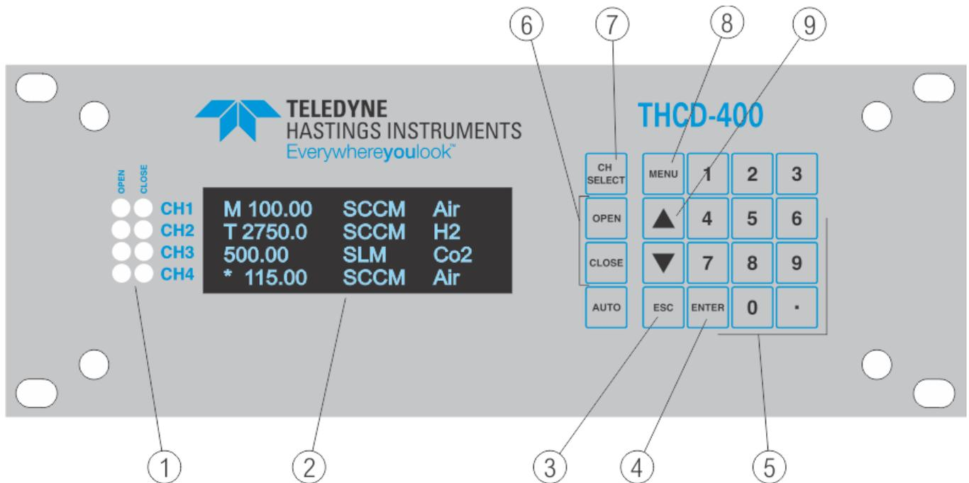
**1. ANNUNCIATORS:** Displays OVERRIDE signal status of each channel. If annunciators are not illuminated, the Setpoint (Control) voltage is active.
