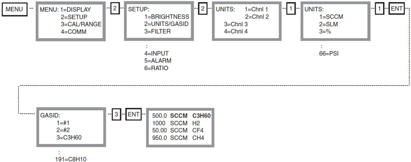
The bold characters shown in the above flow chart indicate the updated Units of Measure and Gas Identifier selected. Note: When the Units of Measure and Gas Identifiers are selected, ENT must be depressed before the selection is made. This is because it may require the inputting of more than 1 digit to make the desired selection.
