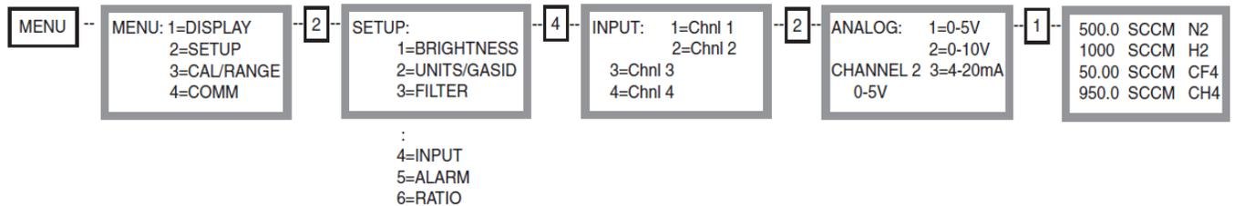
The Input selection sets the full scale input signal and the full scale setpoint (control) signal for the selected channel. The selected channel and the input signal setting that was previously selected is displayed during selection. The factory default is 0-5V for each channel. Any input may be selected for any channel. The instrument compensates for any incompatibilities even in the Master/Slave configuration.
