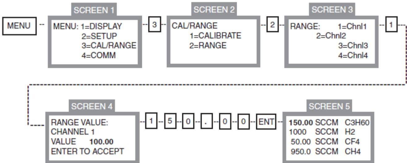
The Range sequence is **not** a calibration sequence. Changing the Range value simply replaces the Range value used during the previous full scale calibration. The analog-to-digital converter data used during the previous full scale calibration is still valid. Ranging is a simple way to change ranges when changing MFC's. It assumes the full scale output voltage of the new MFC is the same as the previous MFC.
